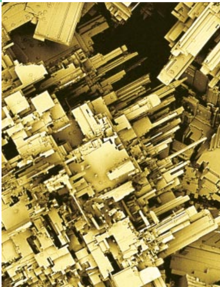
An unusual form of iron pyrites from the Prince Edward Mine. The image, taken on the recently acquired scanning electron microscope, is 500 microns across. The specimen was collected during field investigations into the origins of the gold-bearing mineral veins in the Dolgellau Gold Belt area of Wales.
