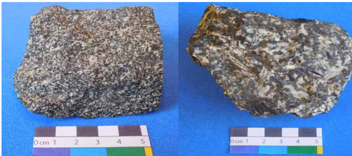
Figure 1. Top left, coarse dolerite, with main components of clinopyroxene (dark) and plagioclase (light) (NMW 51.194.GR.11). Figure 2. Top right, coarser pegmatitic gabbro, with the same mineralogy as the dolerite, from a pod cutting the dolerite. Gimblet Rock, Pwllheli (NMW 30.202.GR.35).
