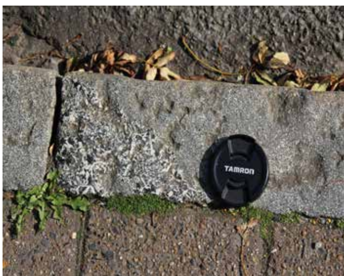
Figure 3. Gimblet Quarry kerb stone, northwest side of Penlan Street, showing dolerite cut by gabbro pegmatite. Photo A. Haycock.
